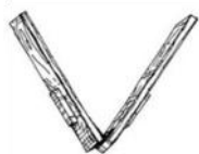
Figure 5. Construct a clapper by hinging together two, 24-inch 2 x 4s. Smack the two sides together.
