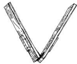
Figure 7. Construct a loud clapper by hinging together two, 24-inch 2 x 4s and smacking them together. (Drawing by Jenifer Rees.)
